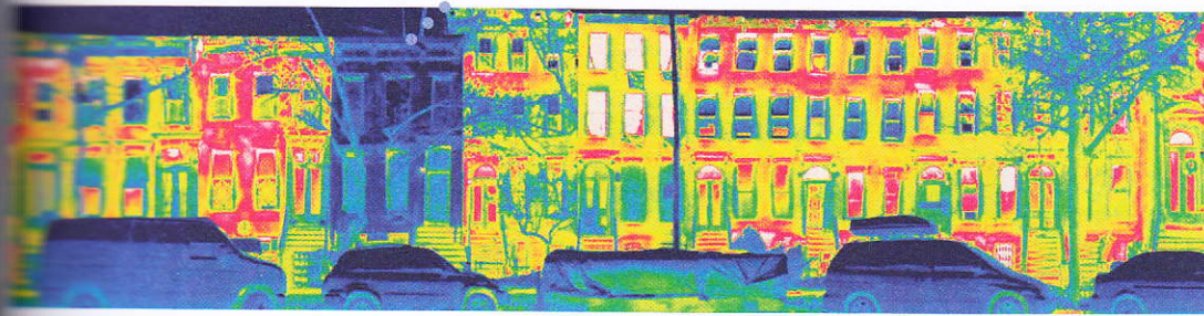
A thermal image of an 1899 Brooklyn brownstone building renovated to Passive House level on a cold evening in New York, USA. The infrared camera shot demonstrates the energy efficiency of this Passive House home compared to the surrounding buildings. 'Tighthouse', Brooklyn, New York, USA by Fete Nature Architecture. Photo: Sam McAfee.
